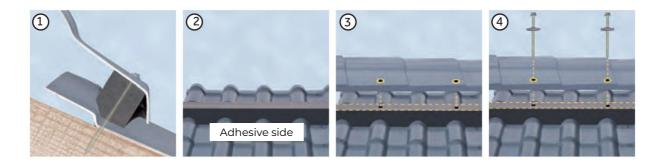
ATTENTION: to optimize the watertight, the hole must be made in correspondence with the upper part of the wave of the sheet and in the middle of the joint (fig. 3).
