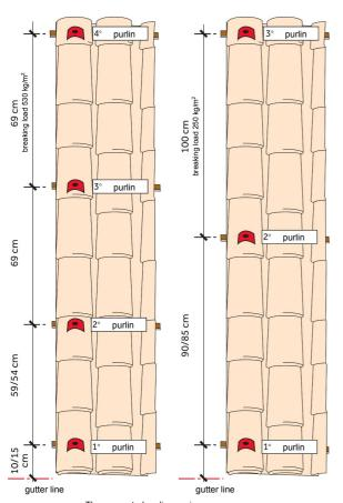
The suggested purlin spacing measures may vary according to installing needs
